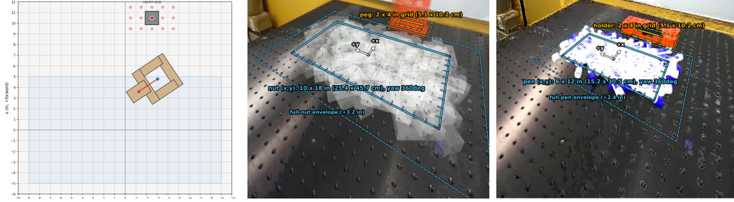
Figure 2: Left: THREAD NUT reset-helper card, the per-episode schematic the operator places objects from (all three tasks in Sec. F.4). Middle and right: initial-state ranges for THREAD NUT (nut pose in white, peg location in red) and INSERT MARKER (pen pose in white/blue, holder location in red), visualized as an overlay of sampled reset poses with randomization-range rectangles and their physical extents annotated. The ROUTE CABLE overlay is in Fig. 1, left.
